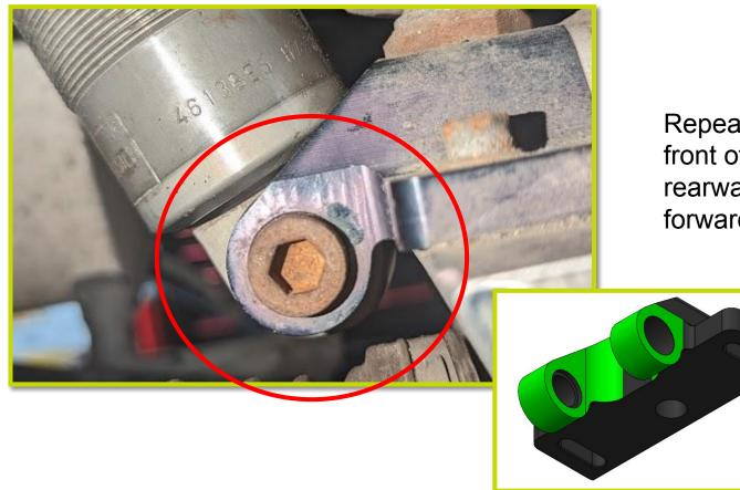
Repeat the same procedure from the front of the rear wing, looking in a rearwards direction, checking the forward-most clevis lug.
