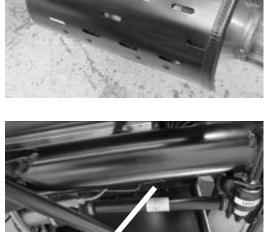
Ensure that the nose cone does not foul against the anti-roll bar.
