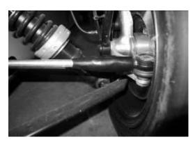
Check all plastic covers are fitted to the front suspension bolt. Also fit to the exhaust mounting bolt heads and (if fitted) rollcage mounting bolt heads.
