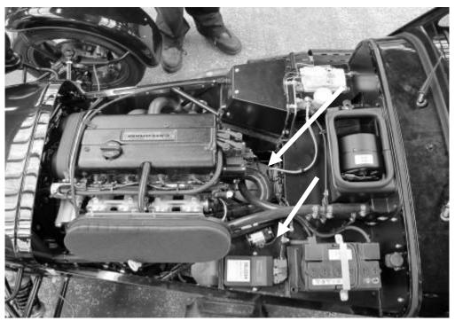
Ensure that the engine bay wiring is secured at least every 300mm or installed in a secure hollow component, eg conduit, and then check that there are no pinch points, sharp edges, etc that wires could rub against, paying particular attention to areas where there is relative movement between components, eg engine to chassis. This applies equally around the car and is not just confined to the engine bay. However, it is essential the engine bay wiring is 'tidy'.
