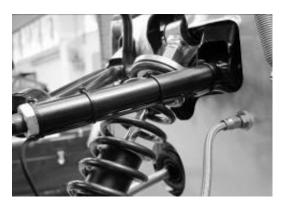
...and that there is some washer pipe where the wire passes into the body work (to protect against chaffing). The pipe can be split with a knife to allow it to be added to the wire.
