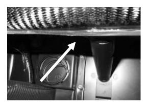
Fit edge trim to the redundant steering column mount on the underside of the dash of the passenger side.
